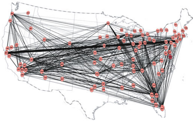
Fig. 2. (Color online) USA air transportation network, with N = 2179 and L = 31326 .
