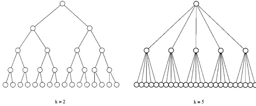
Fig. 5. The left-hand side tree ( $k = 2$ ) has  $N = 31$  and  $D = 4$ , while the right-hand side ( $k = 5$ ) has  $N = 31$  and  $D = 2$ .
