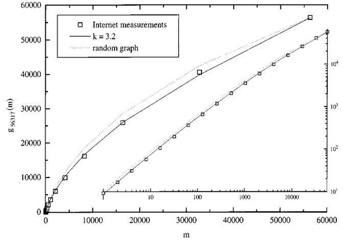
Fig. 7. Internet measurements [13, Fig. 1b] where  $N = 56317$  and  $g_{56317}(m)$ , computed for the  $k$ -ary tree with  $k = 3.2$  and for the random graph on a linear scale. The insert shows the same data on a log-log plot.
