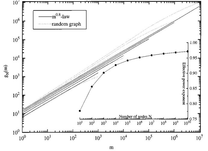
Fig. 4. Multicast efficiency for  $N = 10^j$  with  $j = 3, 4, \dots, 7$ . The endpoint of each curve  $g_N(N-1) = N-1$  determines  $N$ . The insert shows the effective power exponent versus  $N$ .
