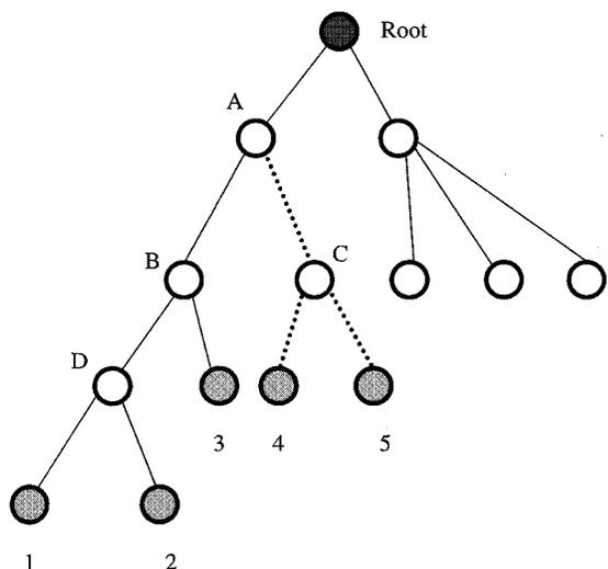
Fig. 2. Multicast session with  $m = 5$  group members where  $Y_5 = 1$  (namely, link C-5). To construct  $Y'_5 = 2$ , the three dotted lines must be removed, and we observe that  $Y'_5 = 2$  (A-C-5), which is referred to as the reduced tree. In this example,  $Y'_5 = Y_4 = 2$  because A-C-4 and A-C-5 both consist of two hops. In general, they are equal *in distribution* because the role of group member 4 and 5 are identical in the reduced tree.
