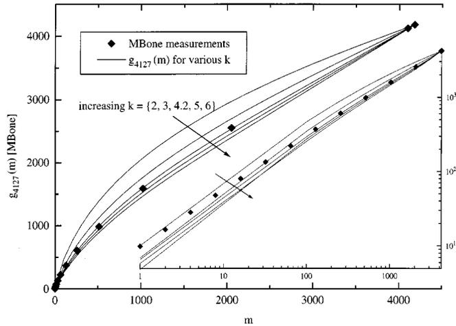
Fig. 8. Mbone measurement from [13] where  $N = 4179$  and  $g_{4179;k}(m)$  computed for the  $k$ -ary tree for various values of  $k$ . The upper curve corresponds to  $k = 2$ ; the curves decrease monotonously for increasing  $k$ . The best fit corresponds to  $k = 4.2$ . The insert shows the same data on a log-log scale.
