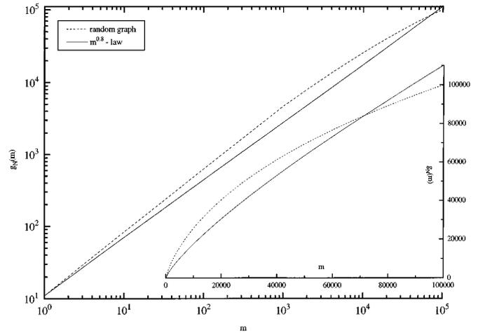
Fig. 3. The Chuang–Sirbu power law versus the exact results for the random graph with  $N = 10^5$  on a log–log scale. The insert shows the same data on a linear scale.
