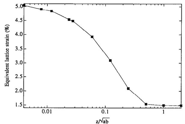
FIG. 3. The equivalent lattice strain  $f_m$  plotted vs the ratio of height  $z$  upon the square of the interface area  $\sqrt{ab}$ .
