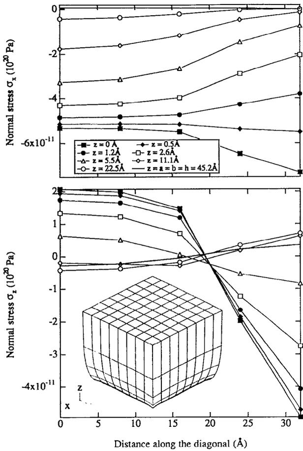
FIG. 1. The normal stresses  $\sigma_x$  and  $\sigma_z$  for various heights  $z$ , as a function of distance from the center along the diagonal to the corner in a parallelepiped ( $a=b=h=45.2 \text{ \AA}$ ), for which the deformed mesh is drawn in the insert.
