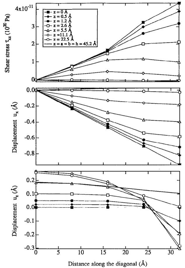
FIG. 2. The shear stress  $\tau_{xz}$  and displacements  $u_x$  and  $u_z$  for various heights  $z$  as a function of distance from the center along the diagonal to the corner ( $a=b=h=45.2 \text{ \AA}$ ).
