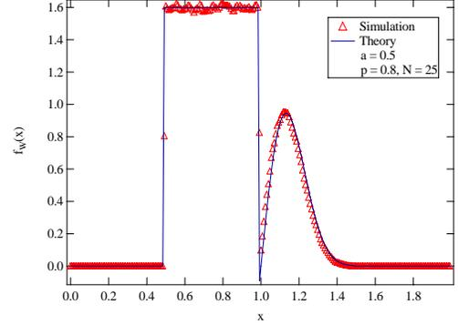
Fig. 2. The pdf of the weight of the shortest path with  $a = 0.5$ ,  $p = 0.8$  and  $N = 25$  computed by (7) and by simulations.
