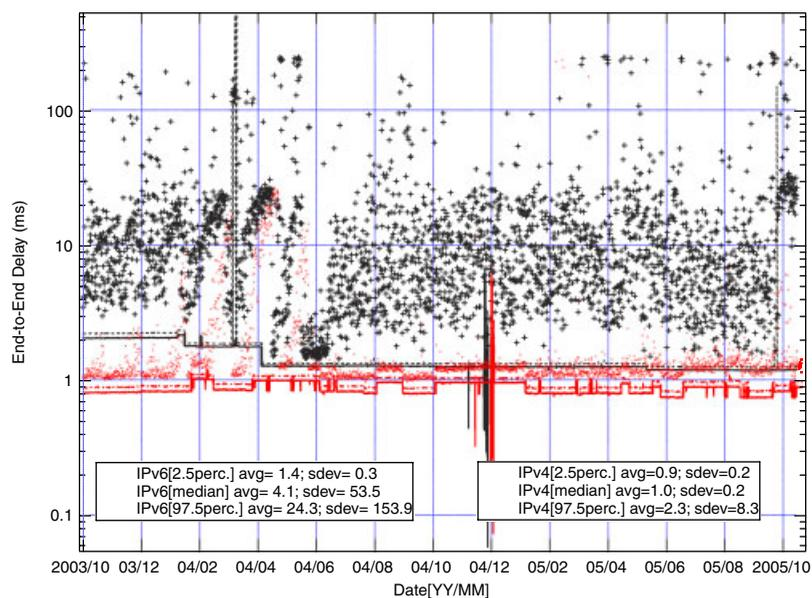
Figure 8. Delay trend of a native IPv6 path over 2 years.
