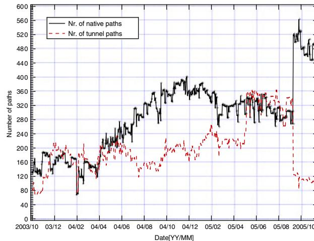
Figure 3. The number of active IPv6 native and tunnel paths over time.
