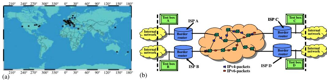
Figure 1. RIPE TTM: (a) location of the RIPE test-boxes and (b) experiment setup.
