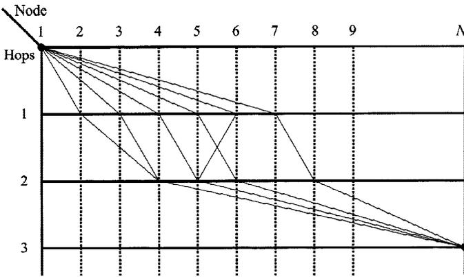
**FIGURE 2.** A sketch of a counting method of paths with three hops.
