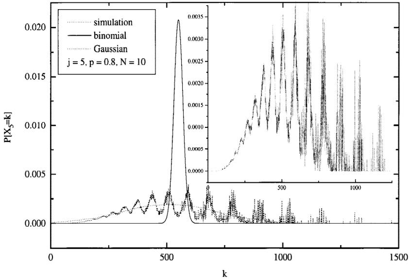
**FIGURE 5.** For  $j = 5$  hops, the width of the Gaussian fit for the simulated results is 410 and is 38.48 for the binomial. The centers are 512.8 and 550.4, respectively.
