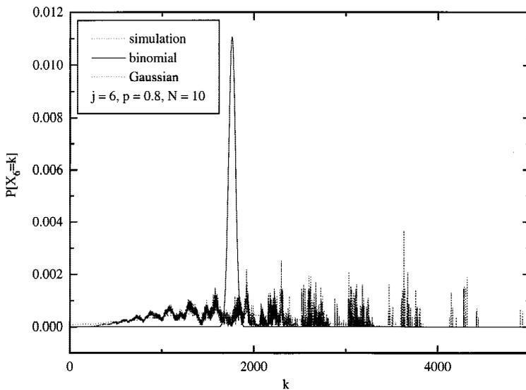
**FIGURE 6.** For  $j = 6$  hops, the width of the Gaussian fit for the simulated results is 1504.7 and is 72.1 for the binomial. The centers are 1584 and 1761, respectively.
