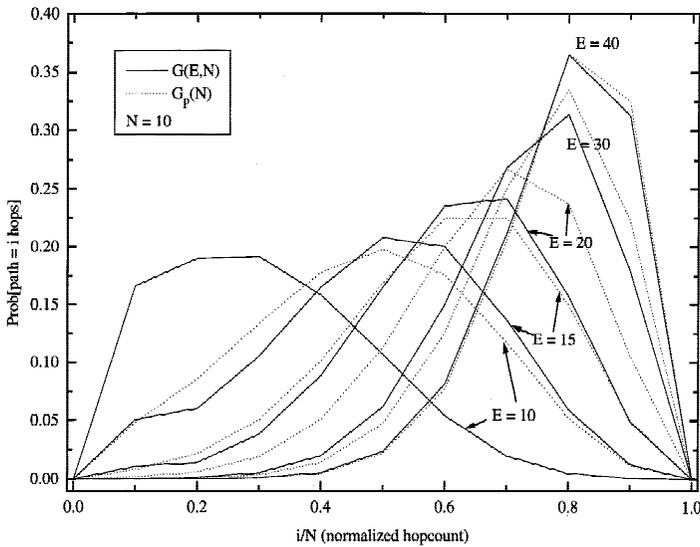
**FIGURE 7.** A comparison of the p.d.f. of the hopcount for  $G(N, E)$  and  $G_p(N)$  computed respectively via the simulations and approximated by the Poisson lower bound. The difference between the Poisson lower bound and the simulation results cannot be distinguished on this graph for  $E \geq 15$ .
