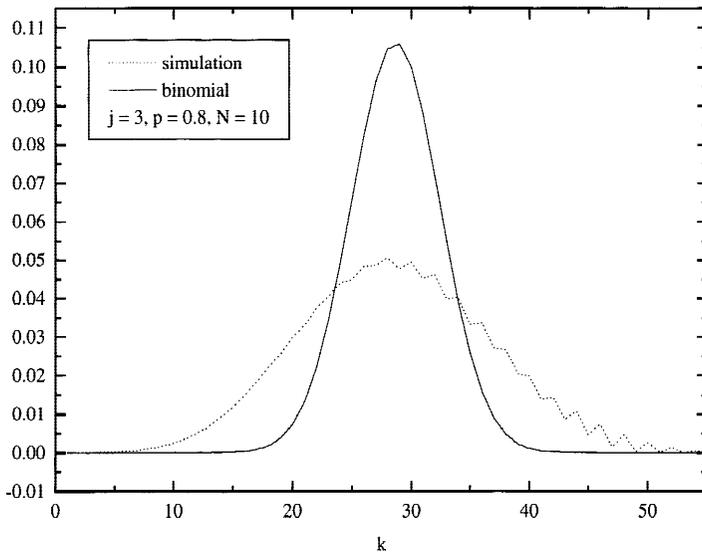
**FIGURE 3.** For  $j = 3$  hops, the width of the Gaussian fit for the simulated results is 16.182 and is 7.5 for the binomial. The centers are 28.42 and 28.76, respectively.
