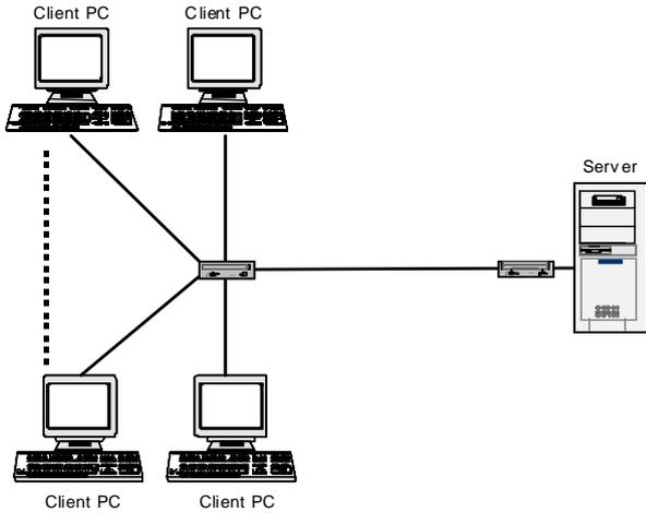
**Figure 2: Client-server architecture for interactive gaming.**
